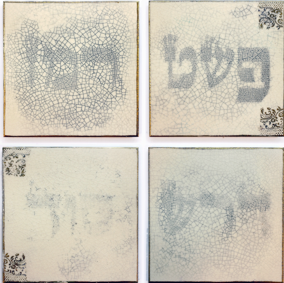
Figure 1: Four ceramic tiles with crackles, displaying a decaying Hebrew text from the Kabala using laser-induced crackles (PaRDeS). From right to left, in Hebrew: Peshat (פשט)—"straight"; Remez (רמז)—"hints"; Derash (דרש)—"inquire"; and Sod (סוד)—"secret." This text is ignorant of the pattern grid and was enforced brute-force, unlike other work presented in this paper.
