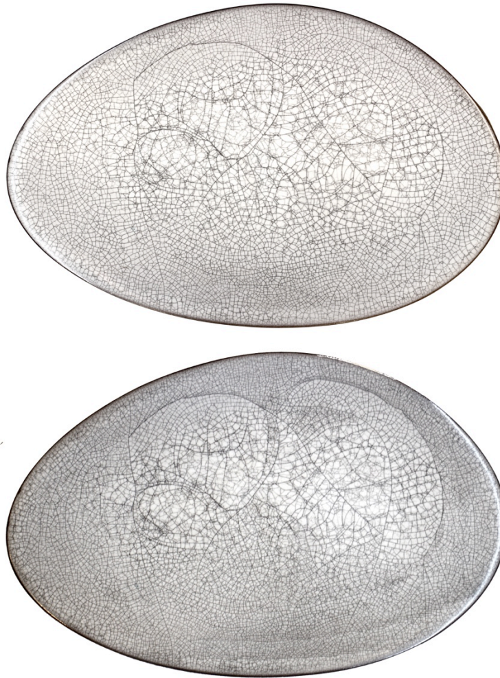
Figure 6: One of the plates from Fig. 5 before and after laser-induced heating results in changes of crackle density in some areas.
